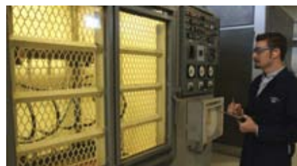
Mega Tested for Superior Quality, Reliability and Value MegaSys hoses meet tough flex-impulse testing up to 1,000,000 cycles
