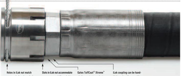
Holes in iLok nut match grooves in female end when fully tightened, allowing passage of a cable to prevent nut from backing off.
